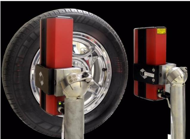
Figure 1: Two WheelWorks HNCA sensors measuring an automotive wheel.
